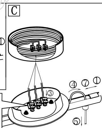
Always keep the fiberglass sleeving between the metal strain relief and the cord to protect the cord from damage
